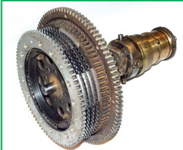
Clutch Bugatti 46 2T 1929 RENSPOINT 12060 - complete refurbishing
